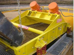
**The ESS Dewatering Screener** operates on the principle of high frequency effect. The dual vibratory motors provide a linear movement to the material to be dewatered.
